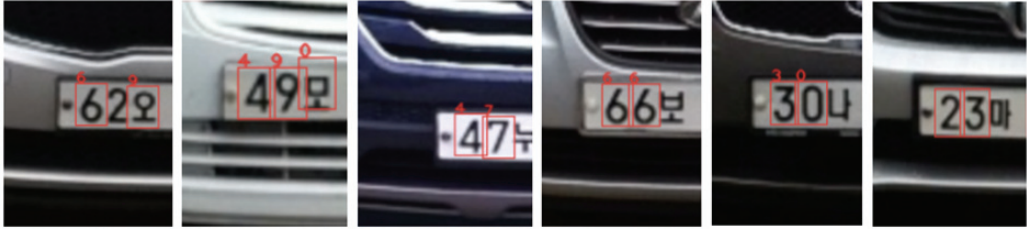
Fig. 7. Digit detection on Korean number plates.
