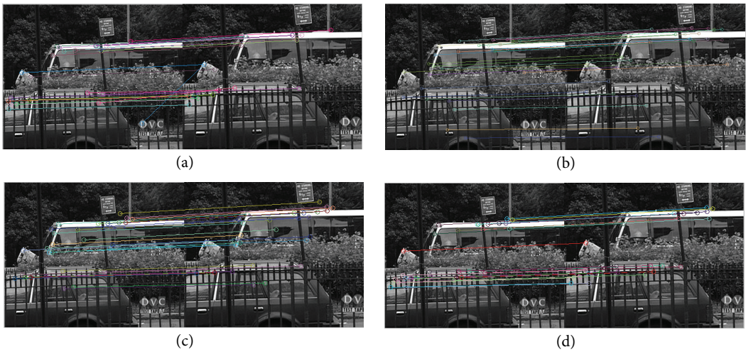
Fig. 2. Feature point matching effect figure for BUS video (the 18th frame). (a) SIFT algorithm, (b) CGO algorithm, (c) Harris algorithm, and (d) SURF algorithm.
